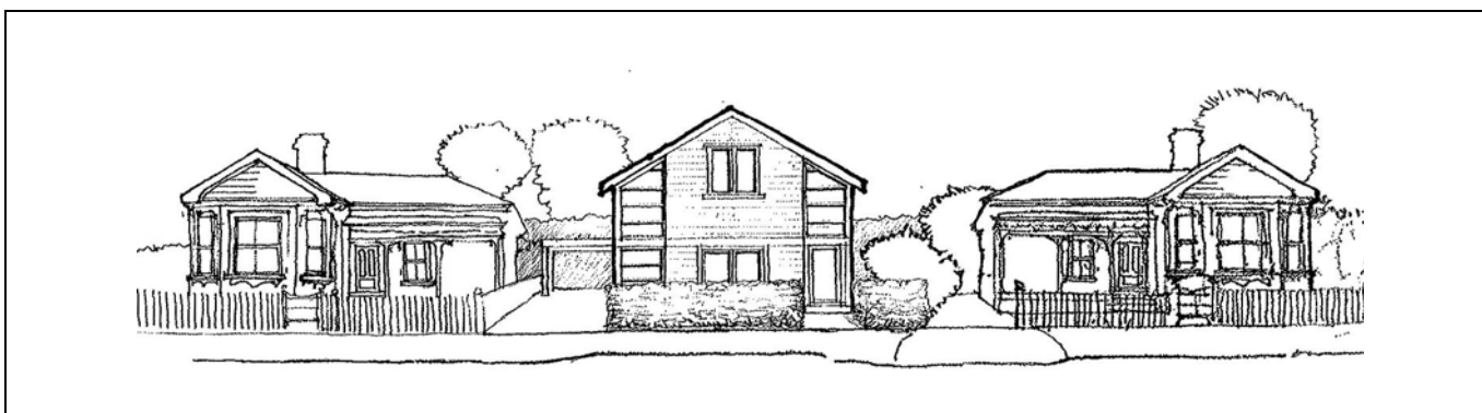
Figure 25. An example of a new house which maintains traditional proportions of elements on the front façade, while incorporating contemporary design ideas.
