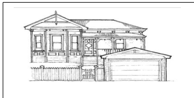
Figure 55: In this the gable on the garage creates an additional level of dominance. It also starts to create a new streetscape of garaging. It would not be consistent with the guidelines.
