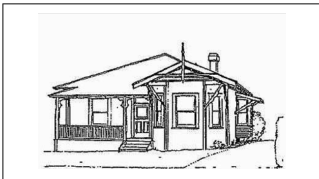
Figure 15: An example of a Transitional Villa. Of note is the lower roofpitch, the verandah beneath the main roof form, and the move towards 'Arts and Crafts' detailing (such as the eaves brackets). The main bay window is once more below the front gable end, but the bay window projecting to the side is now cantilevered in the manner of the later bungalow style.
