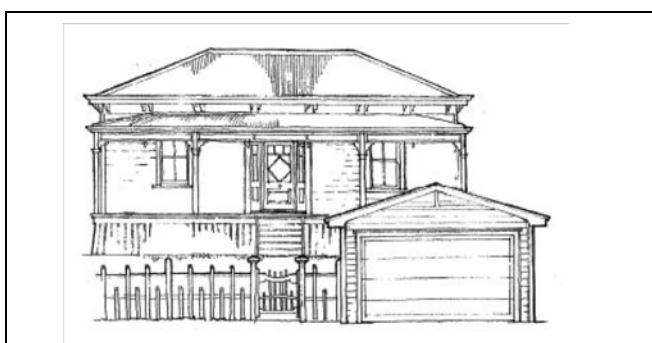
Figure 54: In this the gable on the garage creates an additional level of dominance. It also starts to create a new streetscape of garaging. It would not be consistent with the guidelines.
