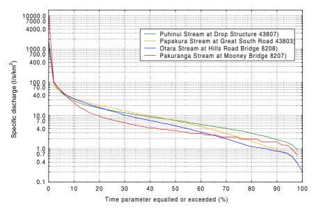
Figure 10.6: Flow duration curves for four Auckland Central area surface water catchments..
