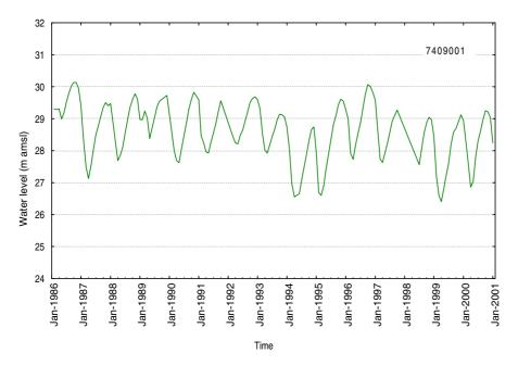
Figure 10.11: Groundwater level record at Burnside Road (7409001) monitoring bore.
