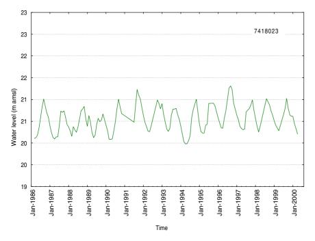
Figure 12.10: Kaawa Aquifer groundwater level record at Batty Road (7418023) monitoring bore.
