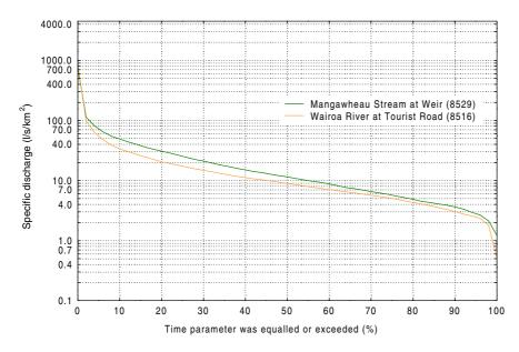
Figure 11.6: Flow duration curves for two Hunua area surface water catchments.
