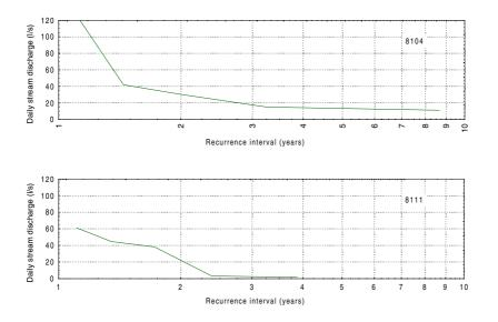
Figure 10.7: Low flow frequency plots at Motions (8104) and Meola (8111) flow monitoring sites.
